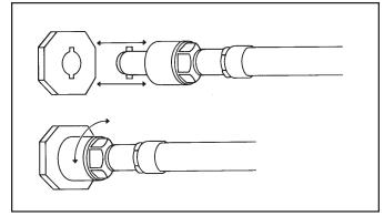
Figure 7. Remove Quick Disconnect
